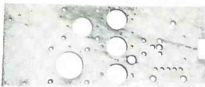
Finished aluminum chassis which has been hard-anodized to give insulating surface. Bare metal is left exposed in strips on sides for grounding purposes
