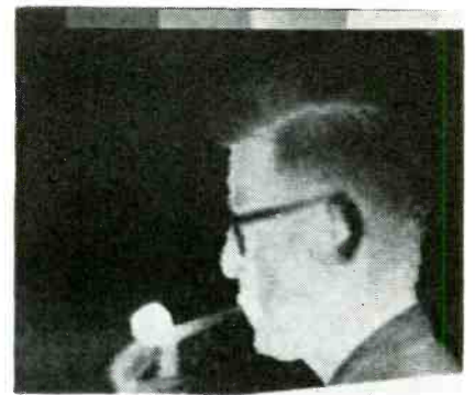
Temperature photo of man with pipe. Gray scale at top compares to temperatures of (l to r) 75.2 F, 77.4 F, 79.5 F, 83 F and 86.5 F
