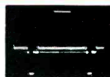
WHITE WINDOW LOW & HIGH FREQUENCY CHARACTERISTICS. Determine ringing, smears, steps, low frequency tilt, phase shift, mismatched terminations, etc. in TV signals or systems.
