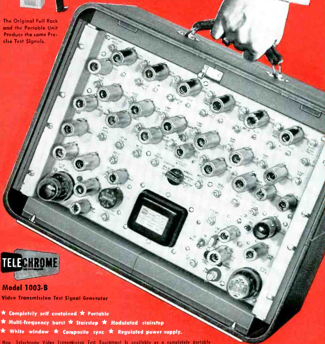
STAIRSTEP SIGNAL modulated by crystal controlled 3.579 mc for differential amplitude and differential phase measurement. Checks amplitude linearity, differential amplitude linearity and differential phase of any unit or system. Model 1003-C includes variable duty cycle stairstep (10-90% average picture level).
