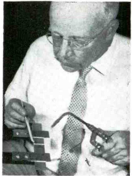
After heating uncleaned aluminum with ordinary torch, just a wiping stroke with stick of new zinc-base alloy solder is enough to give perfect tinning
