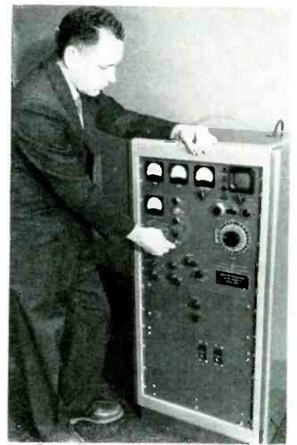
The three sub-units of the suppressed-carrier 100-w transmitter are shown cable-connected for bench testing
