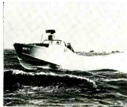
Modified civilian search radar will provide Navy with low-cost all-weather guidance for small amphibious craft
