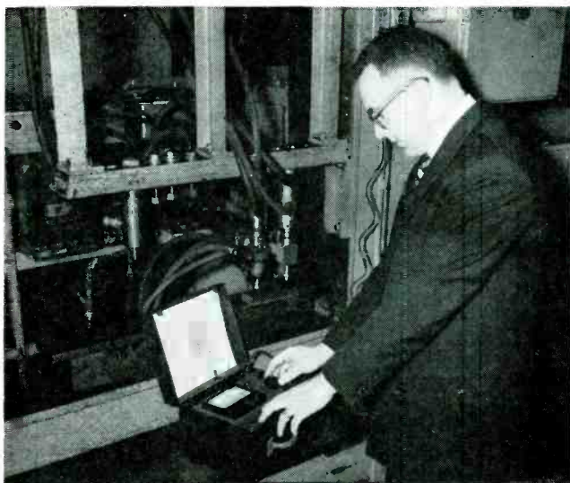
Engineer calibrates resistance-welding current meter. Direct-reading feature permits operation by nontechnical personnel
